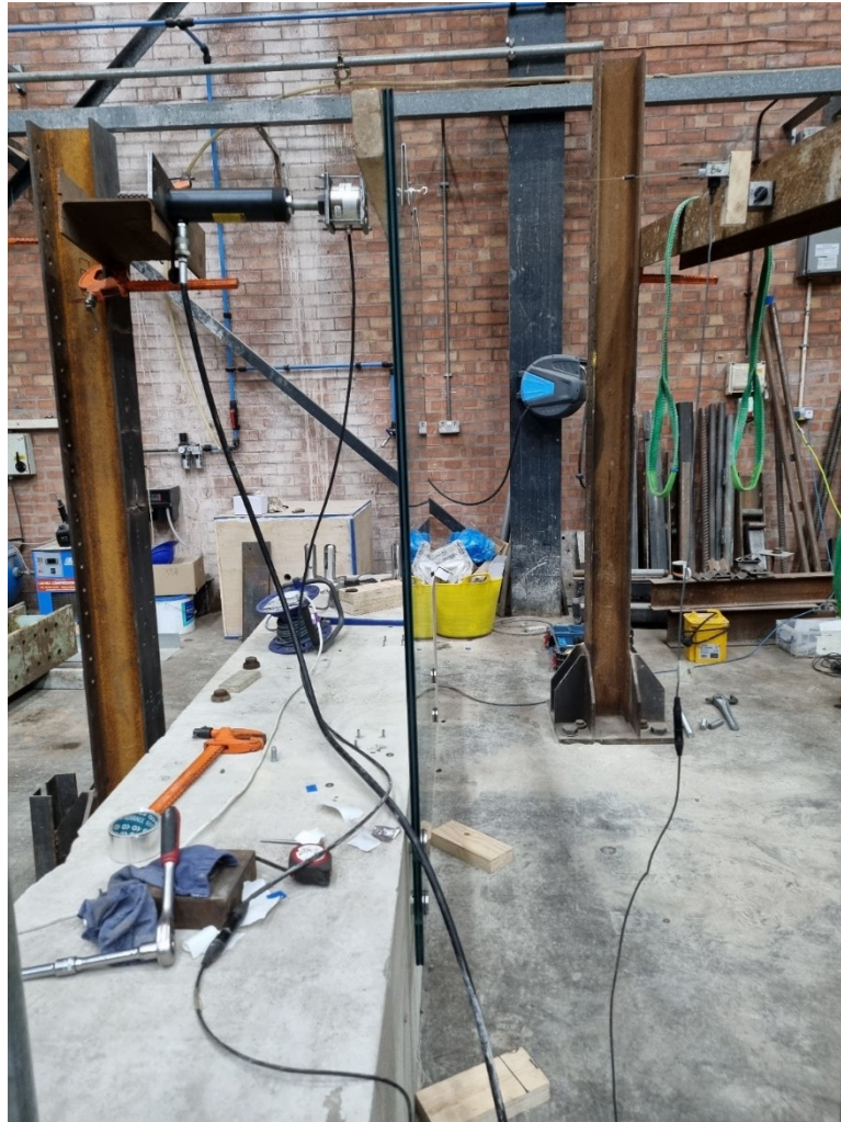
Plate 1 - Typical Specimen Configuration Facia Mount
